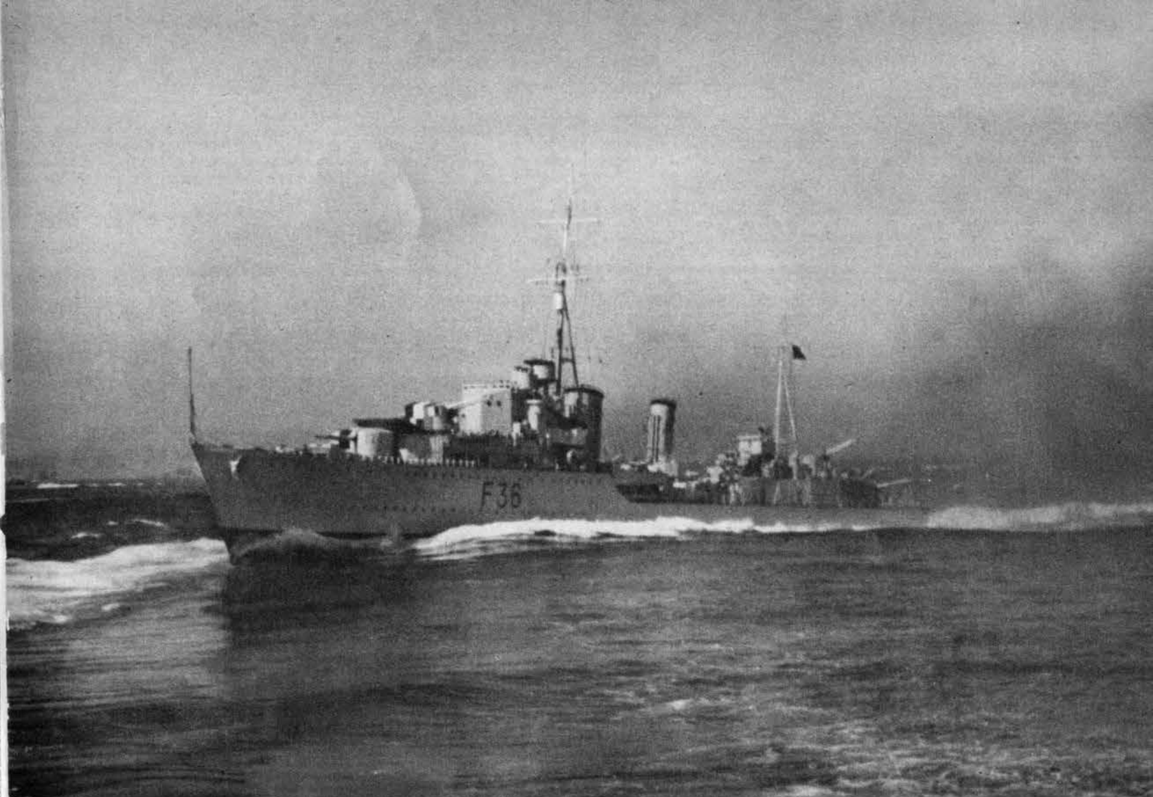
more rake, and bridge shows some streamlining. Mainmast is removed in refitted versions.
